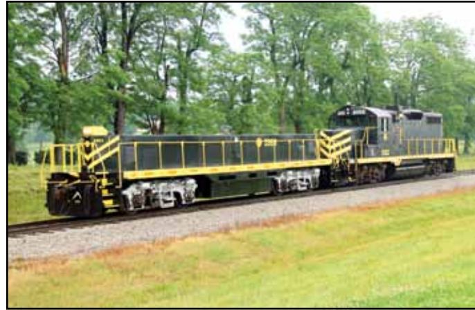
Rail slugs help reduce diesel fuel usage and provide additional pulling power.
